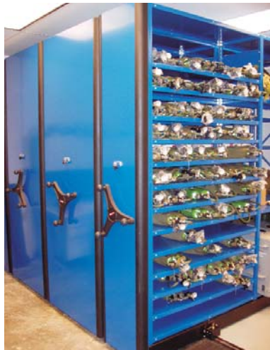
A Mobile Aisle System at Camp LeJeune stores parts, supplies and air tanks in a condensed efficient system.
