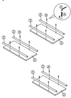
Place Part# 3 on Part# 2 and screw it in. Insert screw (Part A) only halfway in order to leave space for the shelves (Part# 2) to fit on Step 3.
