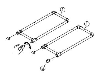
Attach Part B onto Part# 1, then turn it clockwise and tighten it sufficiently.
