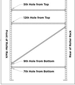
Side supports drop into teardrop shaped holes and are tightened with a 9/16" wrench.
