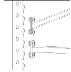
Beams drop into place. Set elevations per included drawing. Install Span-Track per the separate installation sheet.
