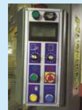
PLC Control With LCD Display
