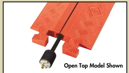
Linebacker GP 1 Channel Features 1-1.25" x 1.25" channels Load capacity: 11,700 lbs./tire, 23,400 lbs./axle. Length: 36"
